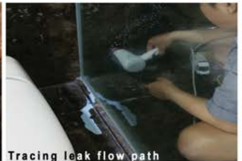
Tracing leak flow path
